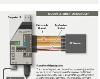
forwards the PPM signal via USB to the computer.
